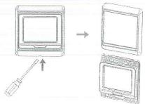
Take the backing plate apart according to the following diagram.
