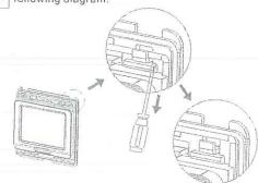
Mounted the backing plate in the wall socket by screwdriver.
